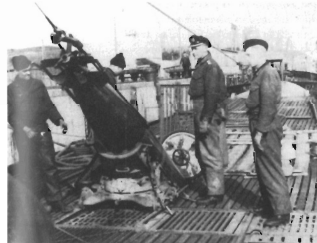
BELOW A G7a torpedo being loaded into a Type IX U-boat.
