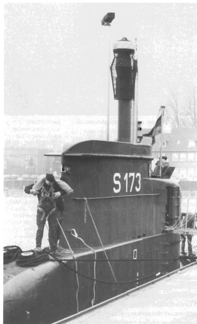
U-Schürer with radar mast, schnorkel and periscope extended. The man standing aft of the conning tower, below, gives a good idea of scale and shows how low the conning towers of these two Class 202 boats were.
