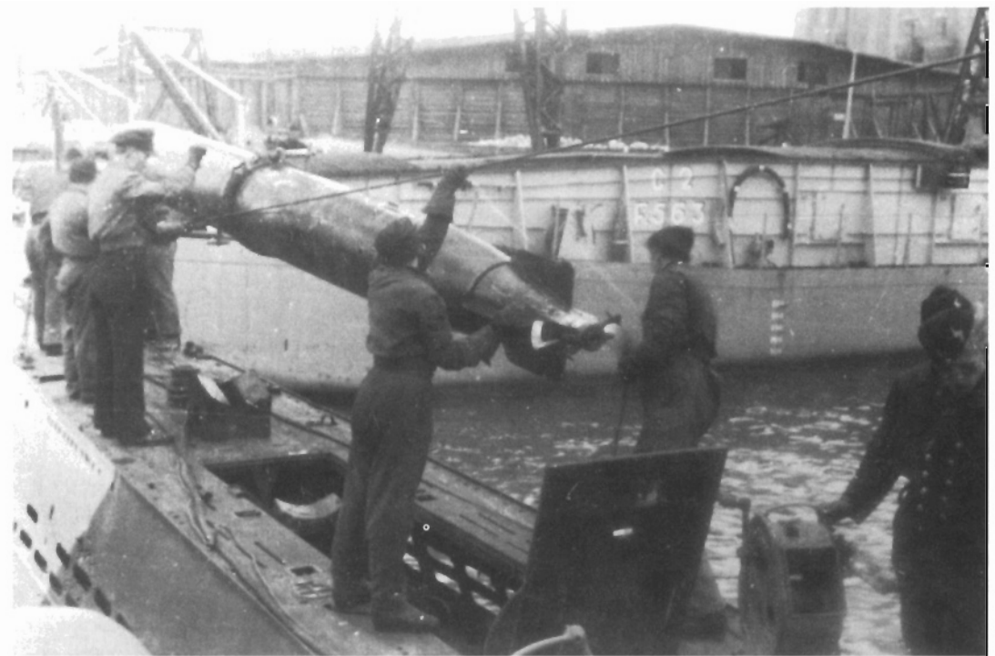
RIGHT A G7e torpedo being loaded into a Type II U-boat. These boats were so small that there was not enough room between the conning tower and the torpedo tubes to slide a torpedo in, and therefore they were loaded backwards, with the torpedo being slid in tail first before being lowered and pushed forwards into the tubes.
