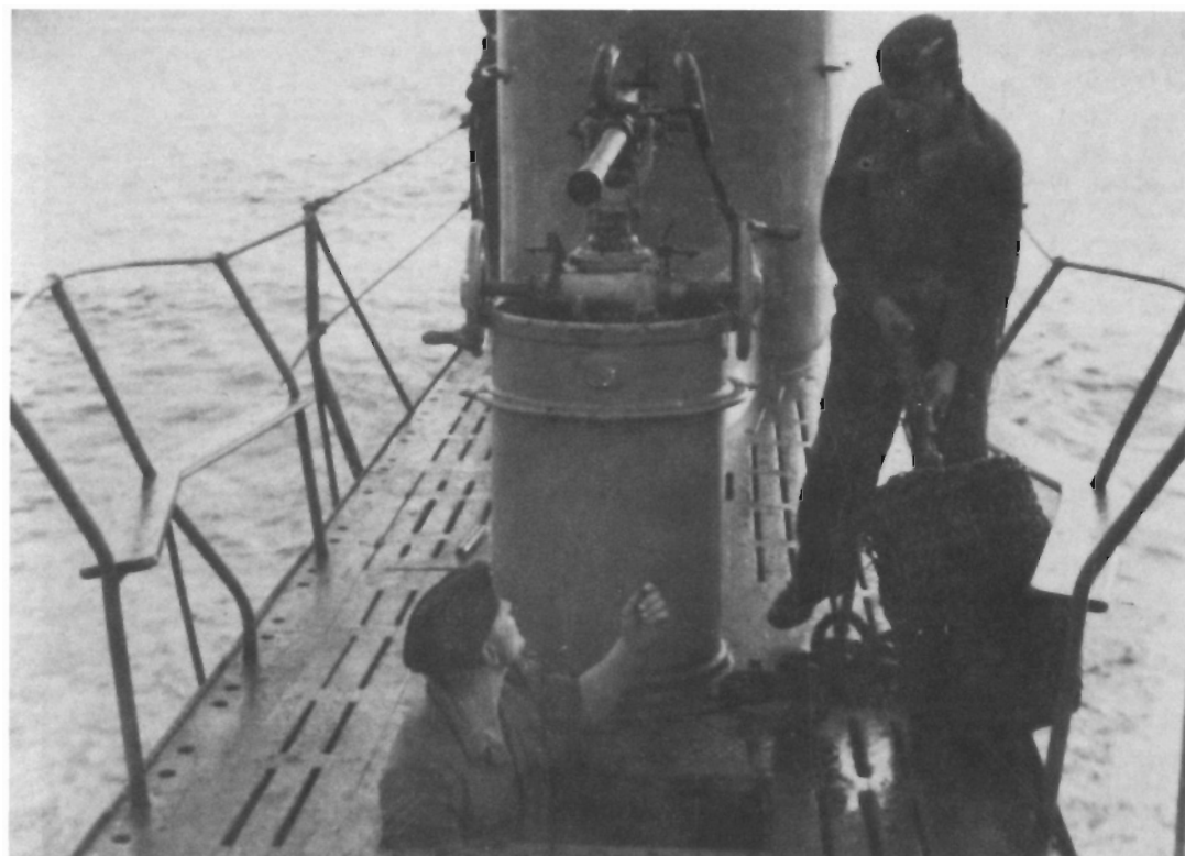
U59, a Type IIC, with 20mm gun on top of the cylindrical mount. Since the man on the right is handling fenders, it looks as though the boat is in port. Ropes and fenders would normally have been stored in lockers between the upper deck and pressure hull. Although there were a variety of different mounts, Type II boats usually carried only a 20mm quick-firing gun forward of the conning tower.
