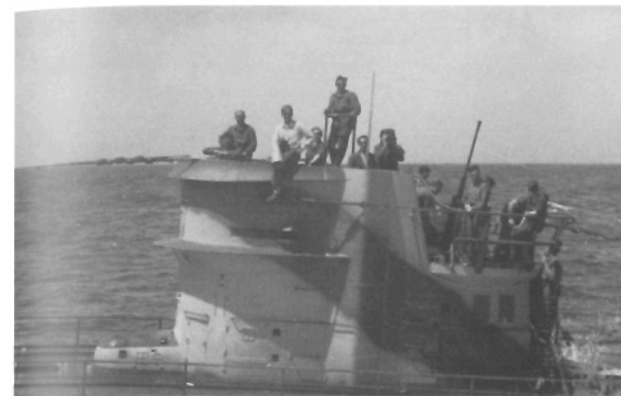
A side view of the early type of conning tower configuration, with a single 20mm anti-aircraft gun on the platform. The man standing on the very top is being supported by a special lookout bracket, which looks 'T'-shaped when viewed from the front or back, but the top was a ring designed to fit around a man's waist.
