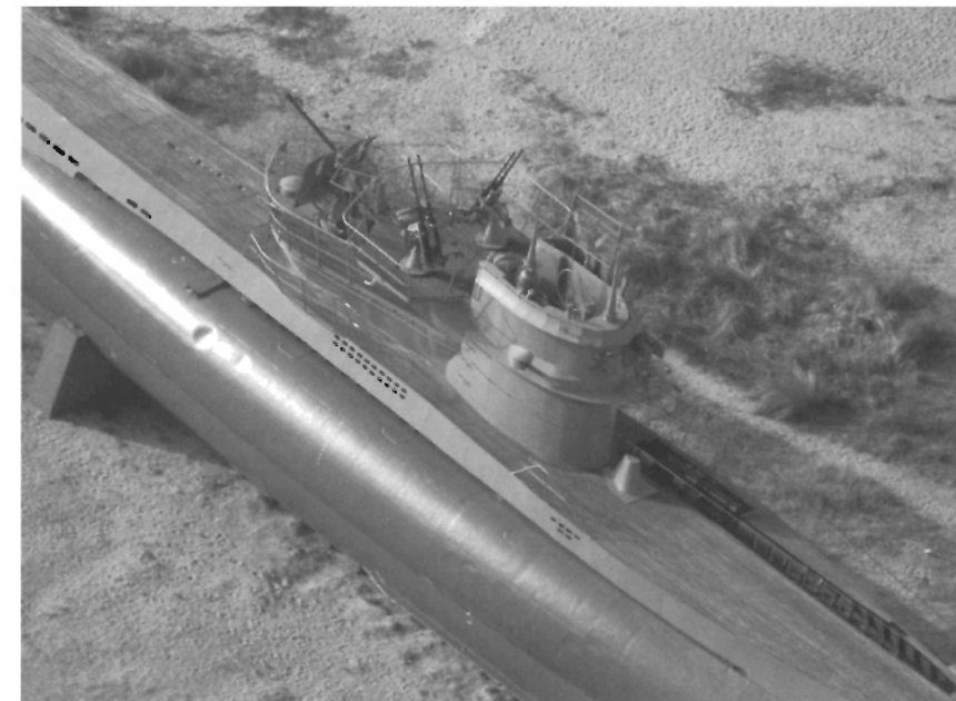
Although this looks like a model, it is U995 photographed from the top of the Naval Memorial to show the later type of conning tower layout.
