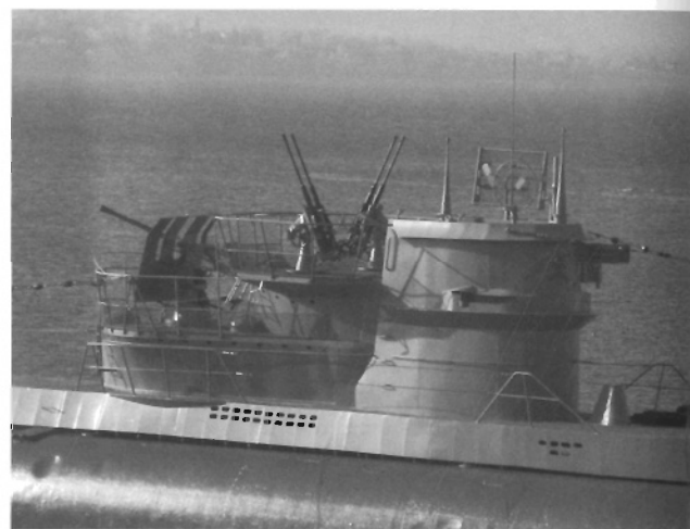
ABOVE The later type of conning tower configuration. The platform by the top of the tower has been enlarged to hold two double 20mm anti-aircraft guns, while the additional, lower platform usually carried either a semi-automatic, single 37mm gun, as shown here, or an automatic quadruple 20mm. There were other combinations, but these two were by far the most common. U995, seen here on display as a technical museum by the Naval Memorial at Laboe near Kiel, was modified to serve in the Norwegian Navy after the war. Once decommissioned, the boat was rebuilt to resemble its 1945 appearance, but by this time it was no longer possible to find all the necessary spare parts. The front periscope, for example, should have had a large head lens for looking at the sky. The bedstead-like structure between the two periscopes is the Hohentwiel radar aerial. This would have rotated and have had a radar transmitter on one side and an enemy radar detector on the other. The circular loop in front of it is the radio direction finder with a rod aerial attached. The bracket for supporting the schnorkel in the raised position can be seen by the jumping wires under the wind deflector by the top edge of the conning tower.
