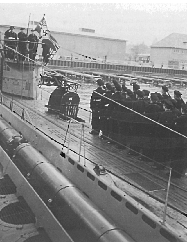
A Type XB minelayer. In the foreground can be seen cargo canisters stored above the mineshafts.
