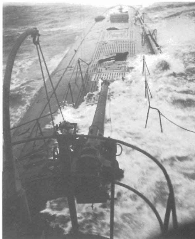
U90 with a more modern, long-barrelled 105mm quick-firing gun forward of the conning tower. Using it in such rough weather, when waves washed over the upper deck, was more than difficult, yet during the First World War nothing was likely to surprise a U-boat on the surface and guns were used successfully under the most appalling conditions.
