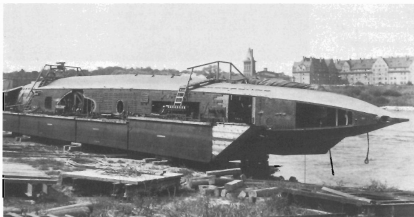
The pontoon for transporting U-boat parts along the Elbe and Danube en route to the Black Sea.
