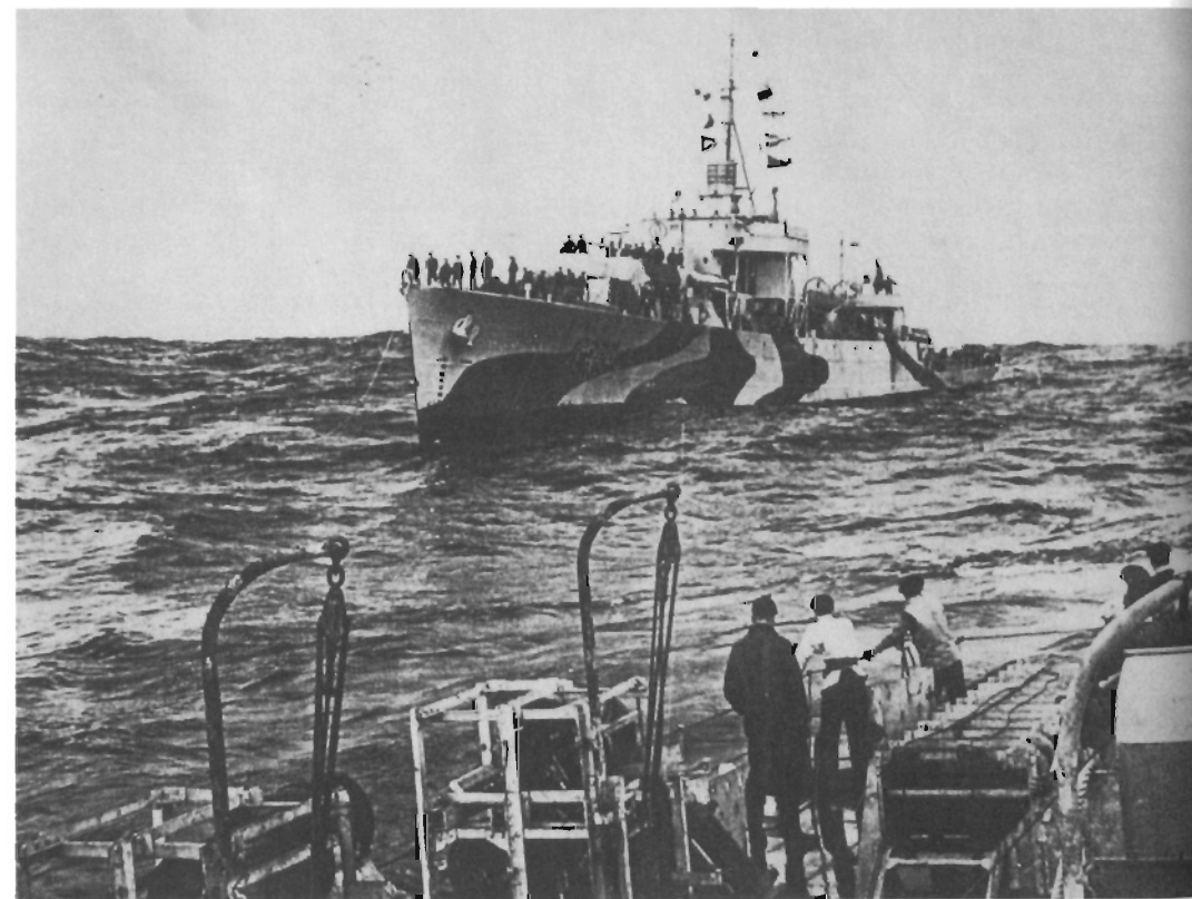
In the foreground can be seen the ready-use depth charge racks and davits for lifting and swinging-out depth charges onto the launch racks on the right. The River-class frigate HMS Swansea is astern.
