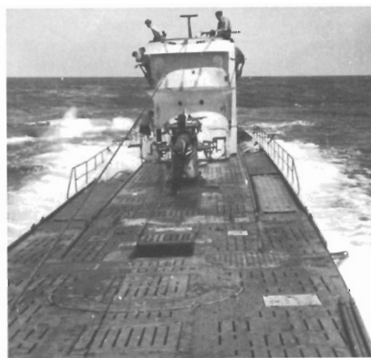
ABOVE U382, a Type VIII C, crashing to the surface with water pouring through the vents from the space between the pressure hull and the upper deck. Such dramatic surfacing procedures were most uncomfortable for the men inside and were usually only performed in an emergency or for the benefit of film cameras.
