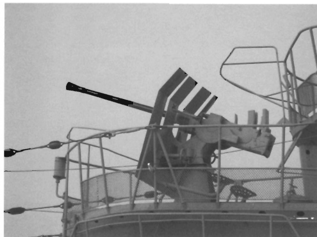
ABOVE The 37mm semi-automatic anti-aircraft gun on U995, which is now open as a museum by the Naval Memorial at Laboe near Kiel. Although this gun was more powerful than the 20mm quadruple, it still did not spit enough punch to deal effectively with modern fast aircraft. The later, twin-barrelled version was much superior, but only a few were installed before the end of the War.
