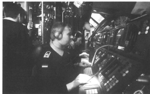
The majority of German submarines are without the all-important 'central control room' for the simple reason that there are only two compartments in each boat. One of these is occupied by the noisy engines and the other by the men. As the boat is so small, there is little distinction between working space and living quarters. This photograph shows what has become of the old central control room; in U28 (S177). It is now called the operations centre or OPZ – Operations Zentrale. Working there is an exceedingly strenuous job, demanding high levels of concentration for long periods, without the opportunity of nipping out into the fresh air for a crafty smoke. Photo: HDW
